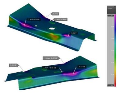
Figure 4: Percentage Reduction in Thickness for DP600 Material (Initial Design)
