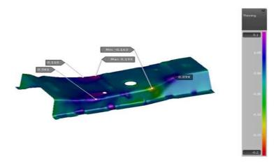
Figure 6: Percentage Thickness Reductions for DP600 Material (Modified Design)
