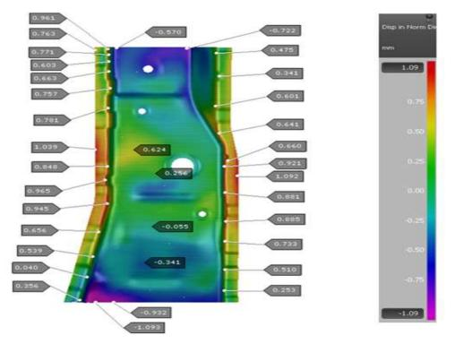
Figure 7: Spring Back at Different Locations for DP 600 Material (Modified Design)
