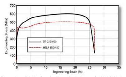
Figure 4: Comparison of the Engineering Stress-Strain Curves for HSLA Steel to a DP Steel
