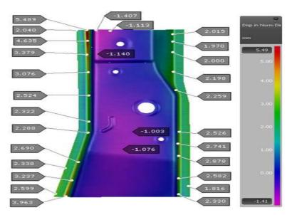
Figure 5: Spring Back at Different Locations for DP 600 Material (Initial Design)
