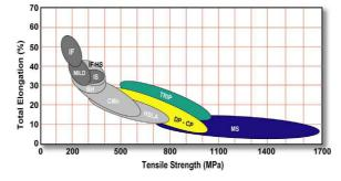
Figure 1: High Strength Steels (In Color) Compared to Low and Medium Steels (Dark and Light Grey)
