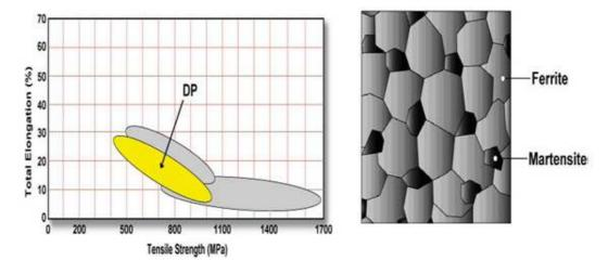
Figure 2: Islands of Martensite in a Matrix of Ferrite
